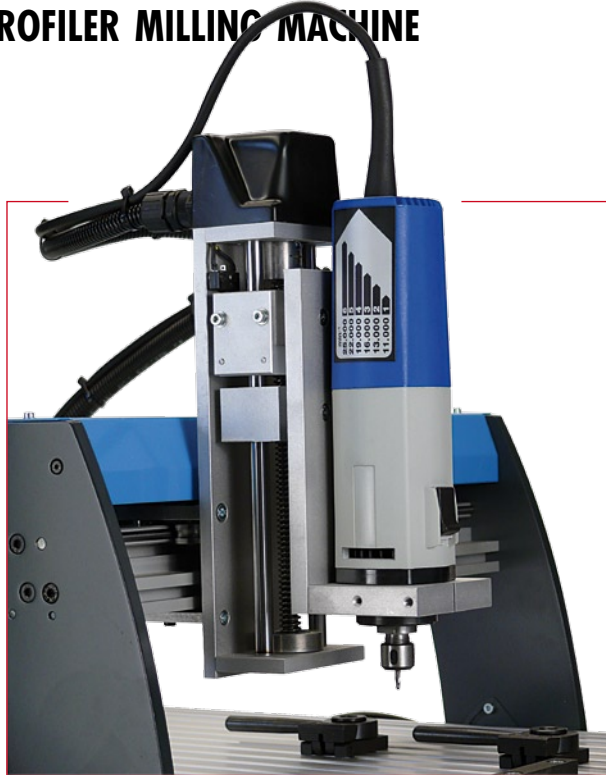
Figure 3. The new Z-axis is more stable and much easier to adjust than its predecessor. In addition it also has a floating head. Here the IACS00 motor from Colinbus is mounted on the Z-axis.
